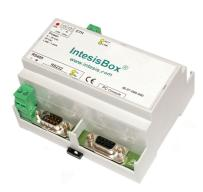
Gateway for monitor and control VRV air conditioning systems of the main manufacturers from Modbus (RTU or TCP) master or client devices (SCADA, BMS, PLC, HMI, TouchPanels...), and in general to monitor/control any BACnet/IP system or device from Modbus.
