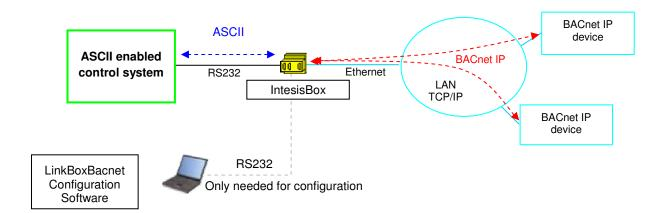
Points in BACnet can be read/written from an ASCII enabled control system using simple text messages. IntesisBox is a BACnet IP client device allowing read/write points of other BACnet IP device(s) connected to a BACnet network, and offering these point's values through its ASCII interface. ASCII interface of IntesisBox uses serial RS232 communication (baud rate configurable). For this application Daikin VRV system must be equipped with Daikin BACnet gateway DMS502B51.
