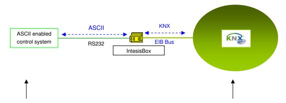
Configurable Control System with possibility to send / receive text messages through RS232 port:
