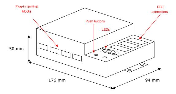
Recommended available space for its installation into a cabinet (wall or DIN rail mounting), with space enough for external connections:
