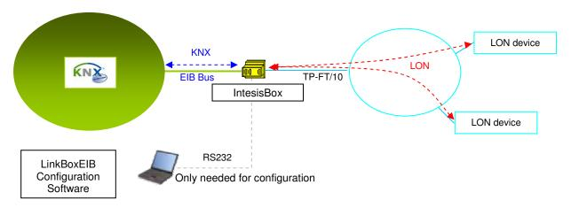
IntesisBox is a KNX device allowing to read/write network variables (SNVTs) of LON devices connected to a LON network, and offering these values through its KNX/EIB interface. SNVT values in LON can be read/write from KNX. Each LON basic data type of a network variable in LON devices can be mapped into an individual KNX group address.
