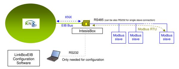
IntesisBox acts as a Modbus RTU master device in its Modbus interface, reading/writing points of the Modbus slave device(s), and offering this point's values through its KNX interface. IntesisBox acts in the KNX side as one more device of the KNX system. IntesisBox's KNX EIB interface connects directly to the EIB bus and is opto-isolated from the rest of the internal electronics
