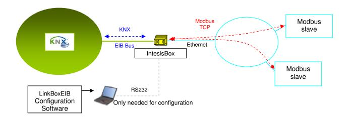
IntesisBox is a Modbus TCP master device that reads/writes points of Modbus TCP slave device(s), and offers these point's values through its KNX interface, acting in the KNX side as one more device of the KNX system. The KNX interface of IntesisBox connects directly to the EIB bus and is opto-isolated from the rest of the internal electronics.
