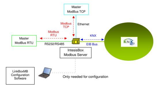
IntesisBox acts as one more device into the KNX system, maintaining always in memory an updated mirror of the KNX points declared in its configuration table, ready to be served to Modbus when requested. *Points in KNX can be read and written from a Modbus master device.*
