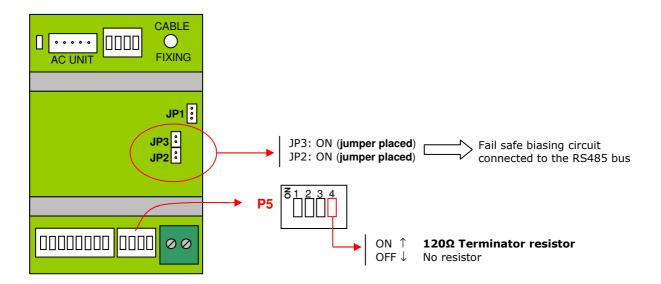
To access to internal jumpers JP2 and JP3, extract the top cover of the interface inserting a small screw-driver or clip in the holes located at both sides of the cover.
