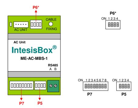
The following table applies for configuration of the interface through these DIP-switches:
